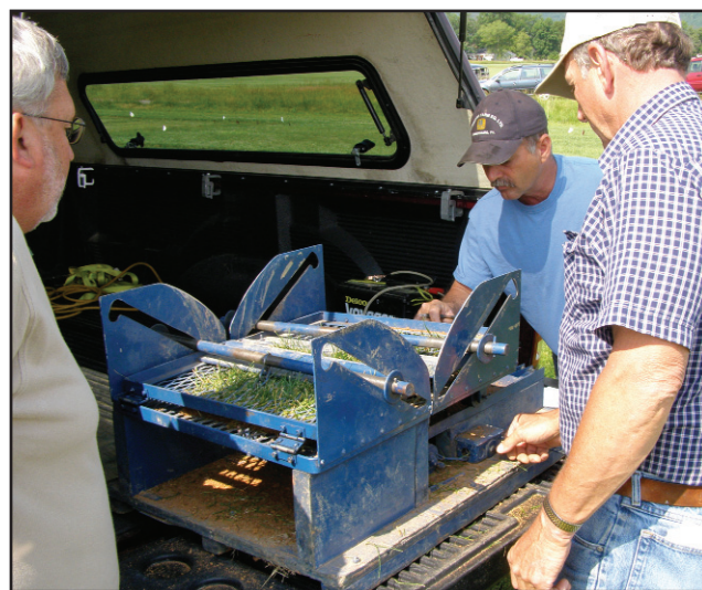
Once the sod is plated and locked down, it is stretched until it tears and the pounds at which it separated is recorded.
