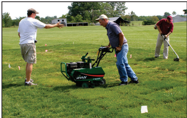
The sod hand harvester cuts a 12 inch swath across each rep in a row.
