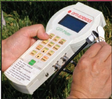
Dr. Xunzhong Zhang performed the photo-chemical efficiency test on all the grasses in the plots. The fluorometer Dr. Zhang is shown using has been improved since the last ratings. We no longer need to lay discs on the plots to block out the sun so that photosynthesis is stopped. Grasses are now placed between the two halves of the black rubber clamp and the laser light is fired through a gun into a target built into the two sides of the clamp.
