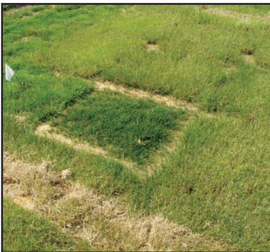
Turf Quality ratings 1 - 9 (9 = ideal turf) Color ratings 1 - 9 (9 = darkest green) Texture Quality ratings 1 - 9 (9 = very fine) Density ratings 1 - 9 (9 = most dense)
